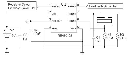
Typical Application Using Self Resonating Piezoelectric Horn
